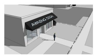
(e) When projecting over a sidewalk or walkway an awning sign shall have a maximum projection of one metre.
