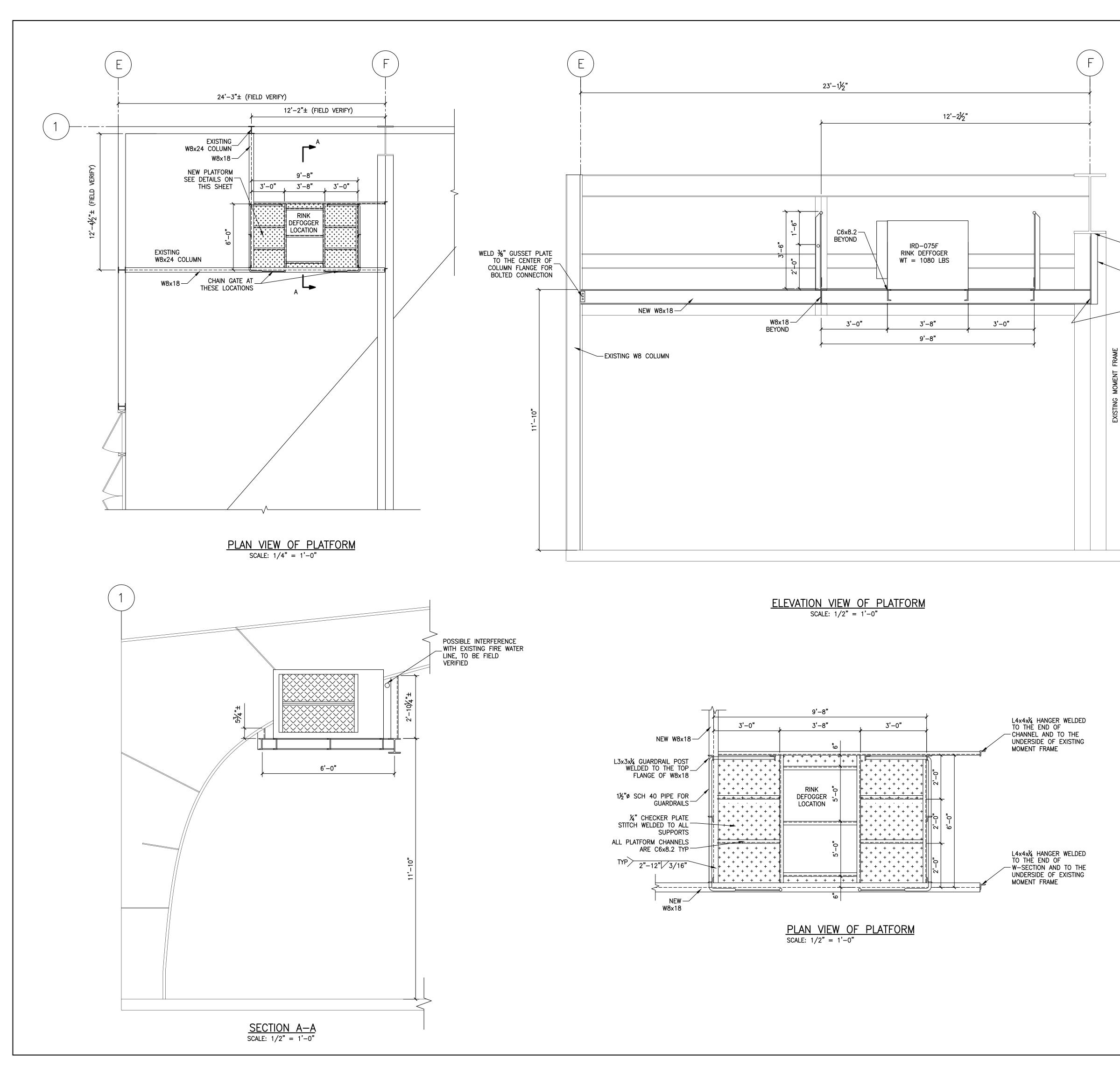
3/16" 3/16" 4x4x<sup>1</sup>/<sub>4</sub> HANGER WELDED TO THE END OF CHANNEL/W-SECTION AND TO THE UNDERSIDE OF EXISTING MOMENT FRAME
