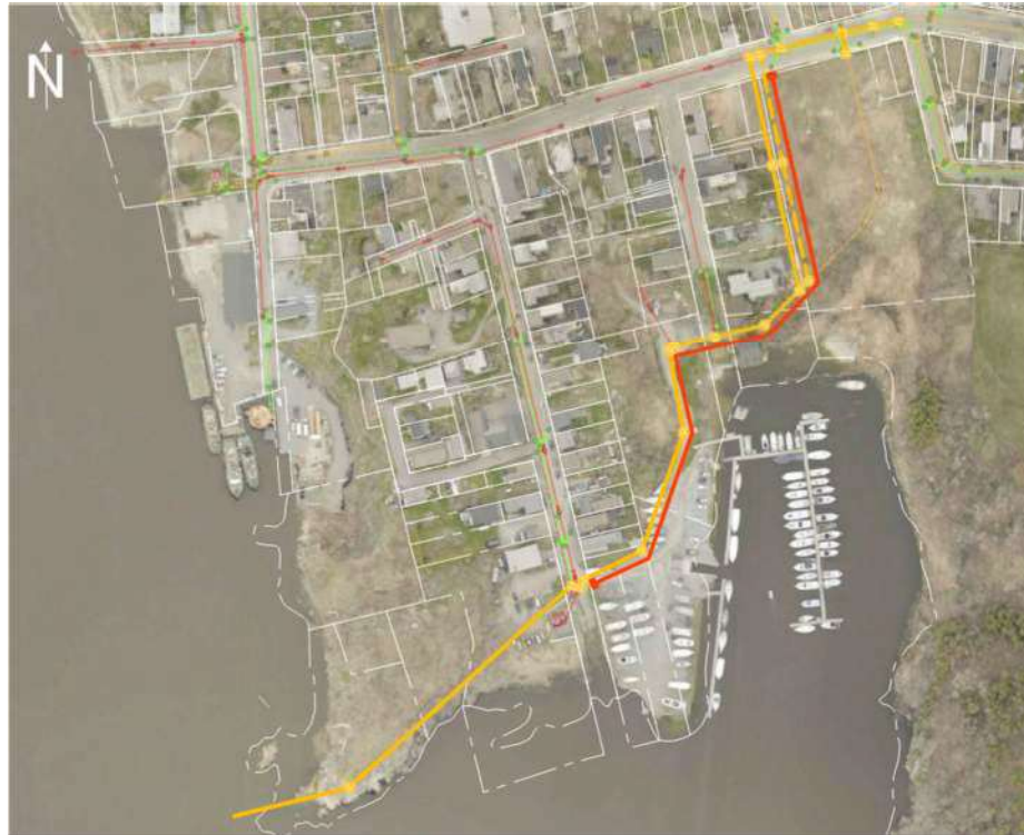
Figure 4: Option 1 – Proposed Sewer Realignment along the West Side of Parcel Identification Number (PID) 00374181
