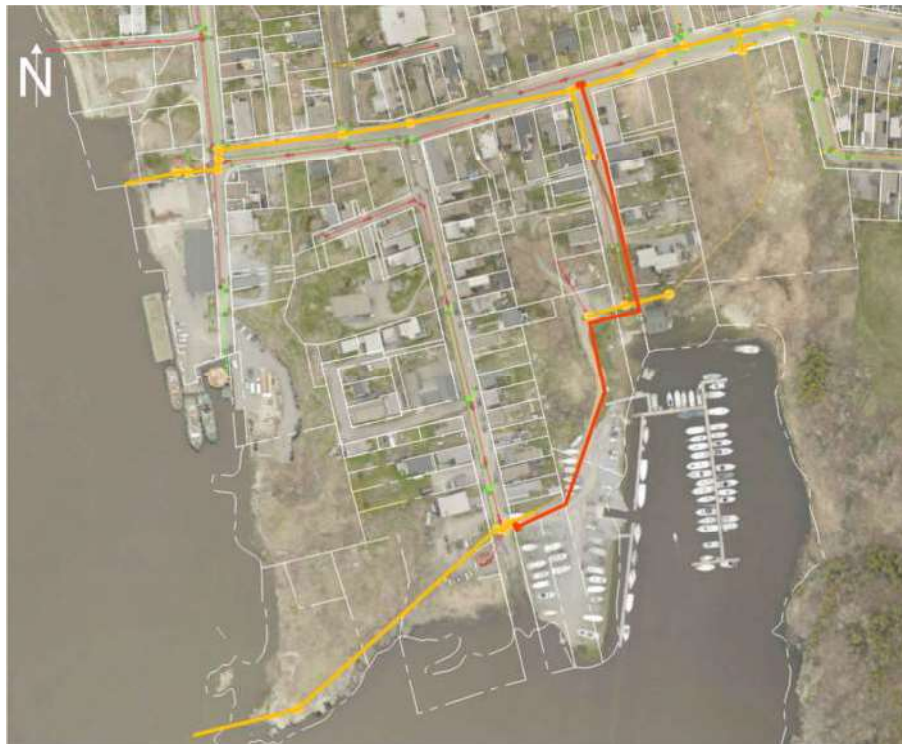
Figure 11: Option 4 – Proposed Sewer Realignment along Main Street
