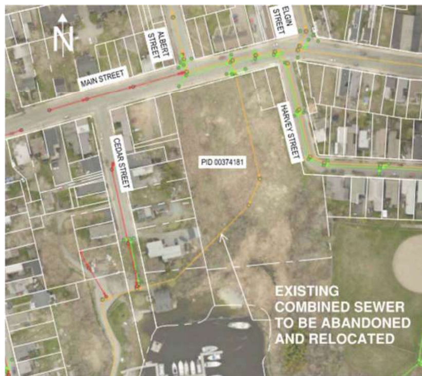
Figure 3: Existing Combined Sewer Requiring Relocation
