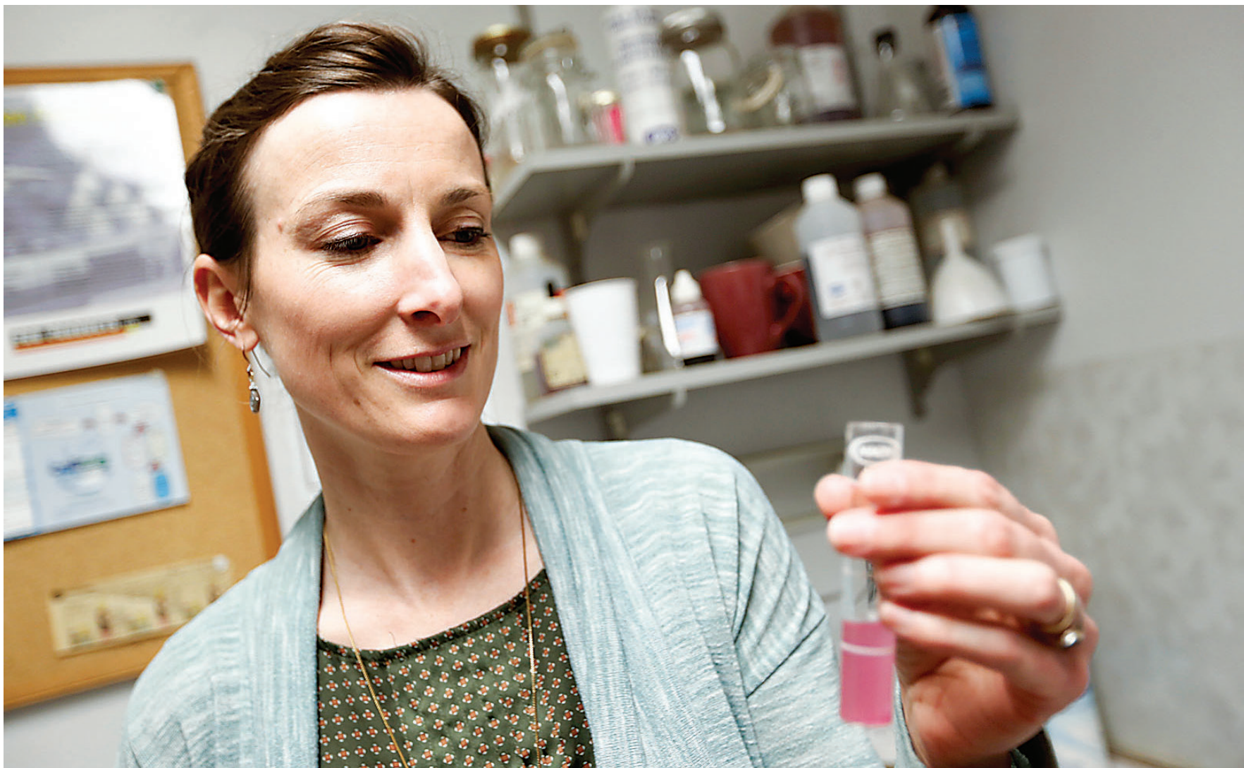
Jennifer Ferris, co-owner of Culligan of Rothesay tests some water in the water lab Thursday. The water has turned pink after a testing chemical was added, indicating that the water is harder than standard. PHOTO: JUSTIN SAMANSKI-LANGILLE/TELEGRAPH-JOURNAL
