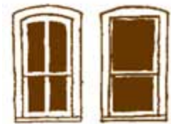
No: Arched top has been removed. Vertical muntin bars have been removed. Original style and proportions have been lost.
