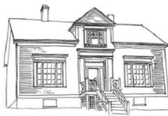
Wood cladding and trim are common in the residential districts. If properly maintained, wood cladding has a long service life. Due to the maintenance they require, wood components are the building features most commonly replaced or altered, but can be easily repaired if properly cared for.
