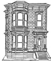
Brick and stone are common cladding materials in Saint John's Heritage Areas. They generally have a long service life, but moisture migration and mortar failure are the leading reason for masonry deterioration. Items to watch for: spalled or damaged bricks and stones, repointing of mortar and sensitive cleaning of stone and brick surface.
